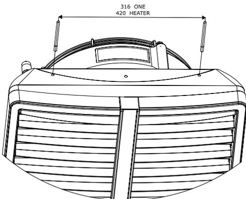
**Installation of mounting pins**
