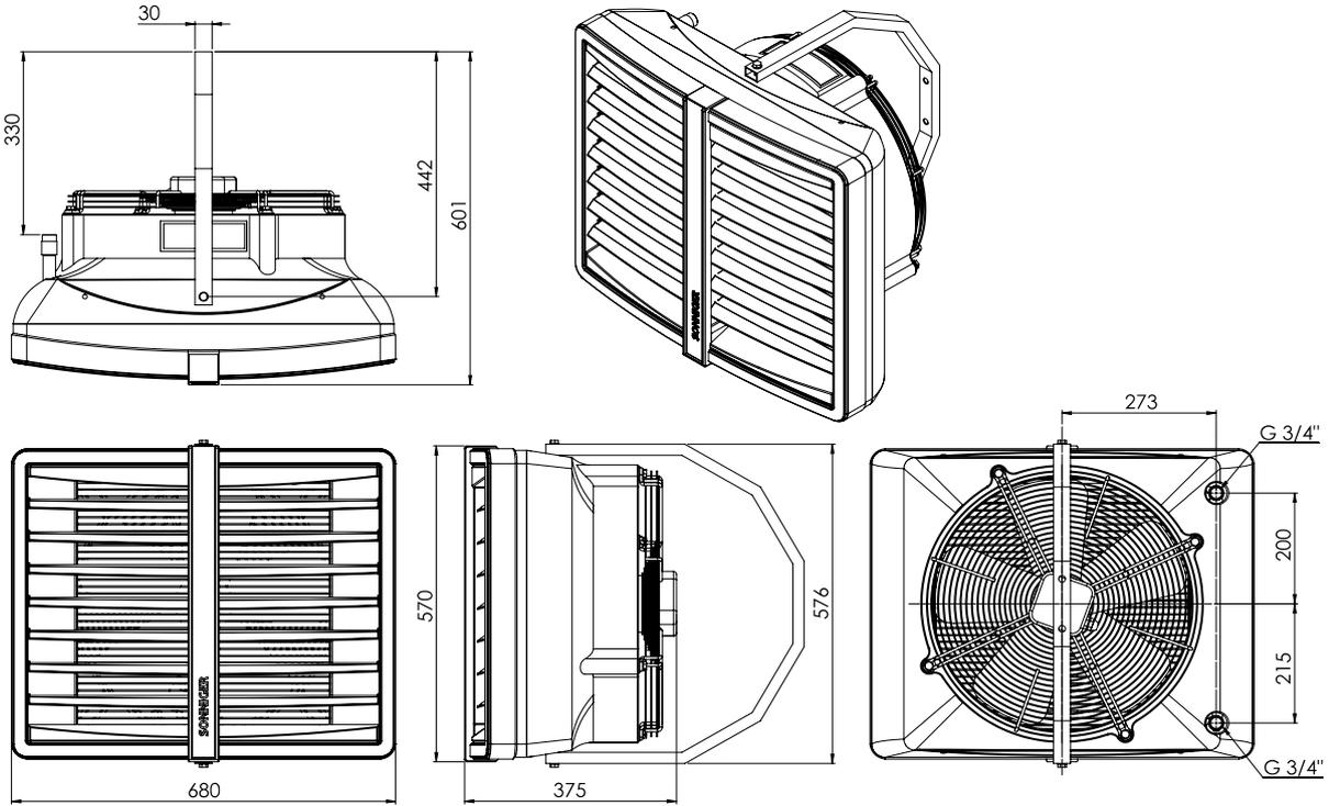
**DIMENSION AND BASIC TECHNICAL PARAMETERS HEATER ONE**
